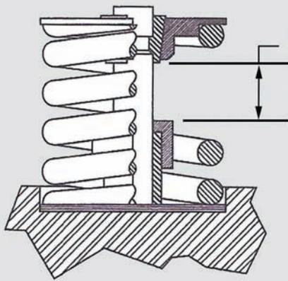
**Valve Spring Retainer to Valve Seal Clearance (0.090" minimum)**
