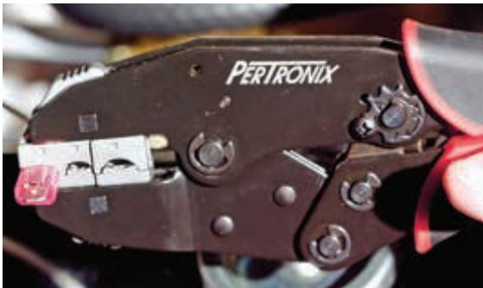
PerTronix’s T3001 crimp tool makes wire terminations simple.
