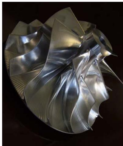
The compressor wheel is intriguing: an embodiment of mathematical complexity and almost supersonic velocity. Operating at the speed of sound, incidentally, would impede performance and be detrimental to NVH (noise, vibration and harshness) requirements.
