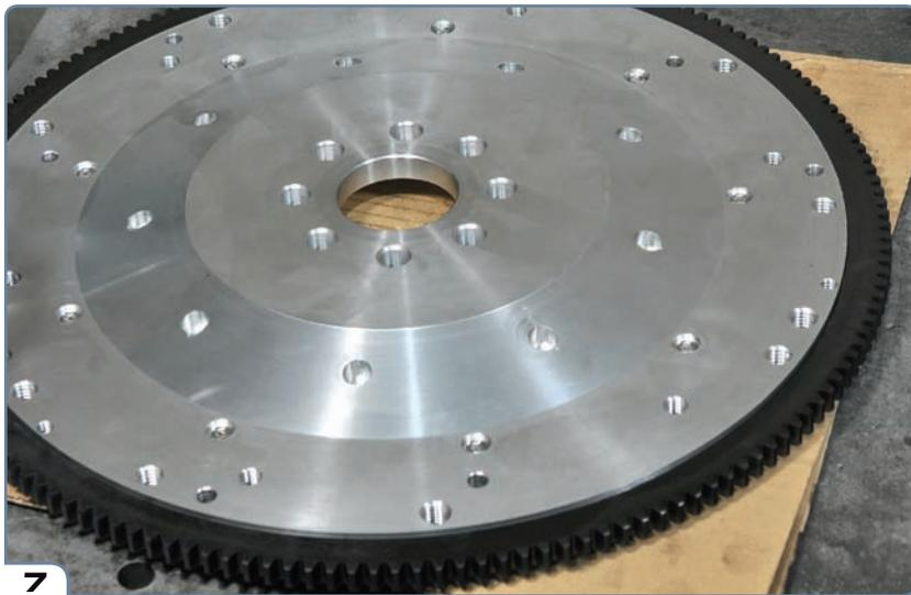
**7** All Ram flywheels are drilled for multiple clutches. Here is an eight-bolt example for the new Mustang, which features holes to accept the original equipment 11-inch diaphragm clutch, the earlier 11-inch three-finger long-style clutch, or the 5-liter 10.5-inch diaphragm clutch.
