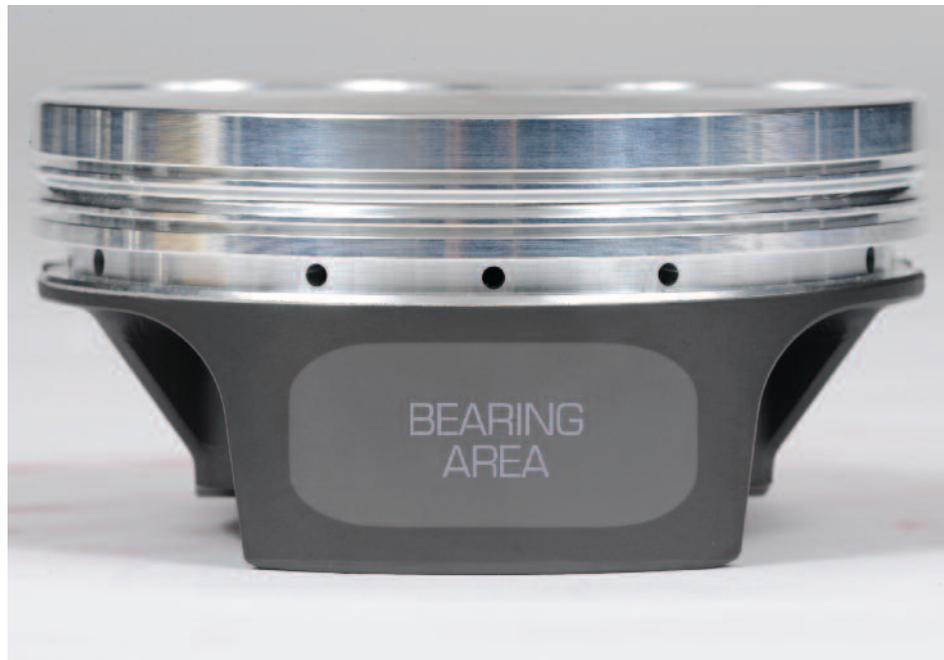
/// A further form of ovality can be found in the middle of the piston skirts. A bearing area rides in the cylinder and is surrounded by a boundary of piston skirt that should not touch the cylinder wall to avoid friction.
