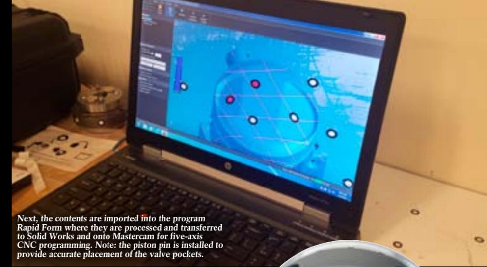
Next, the contents are imported into the program Rapid Form where they are processed and transferred to Solid Works and onto Mastercam for five-axis CNC programming. Note: the piston pin is installed to provide accurate placement of the valve pockets.
