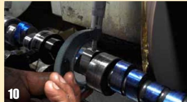
The complexity of modern camshaft lobe profiles means that measuring their dimensions is difficult for the average end user. However, a micrometer can be used to provide an accurate lobe lift figure; here, an inspector checks the overall dimension of a lobe during the manufacturing process.
