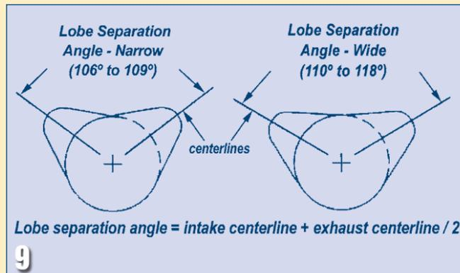
Each camshaft lobe has a center line that runs between the peak of the lobe and the camshaft’s axis; the dimension that exists between the centerline of the intake lobe and the exhaust lobe is expressed as lobe separation angle (LSA). Narrower LSA profiles favor power production in the upper RPM range, while wider LSA promotes smooth idle and low-end torque production.
