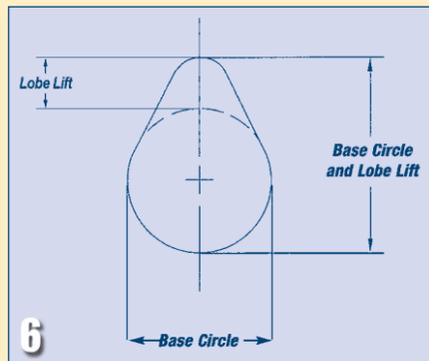
Lobe lift is determined by subtracting the base circle dimension from the figure measured at the peak of the lobe.
