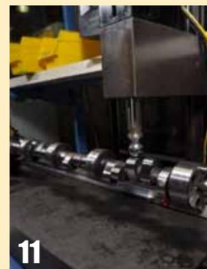
Camshaft manufacturers use equipment that can “read” a camshaft’s lobes to provide all of the critical dimensions as part of the inspection process. This apparatus has been programmed with the cam profiles it will be checking, which it does by running the ball along the lobes, then comparing its findings with the design data. Its duties include measurements of taper, base circle, base circle run-out, toe-to-heel and lobe separation angles. 🛠️
