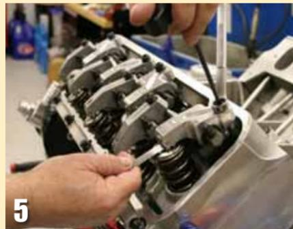
Valve lash measurements on race engines with solid flat tappets or solid roller tappets are often used as a tuning aid—they’re increased or decreased to suit the particular model engine.
