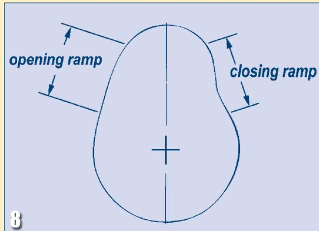
The portions of the cam lobe leading from the base circle to peak lift and then back to the base circle are referred to as the ramps; the term “ramp angle” is used to describe the specific dimensions of the ramps used with a particular lobe profile. An asymmetrical ramp is shown.
