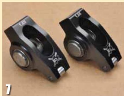
Rocker arm ratios multiply the effect of camshaft lobe lift to yield valve lift. The rocker’s ratio is the distance from the center of its pivot point to its tip (where it exerts force on the valve stem) divided by the distance from its center of pivot
