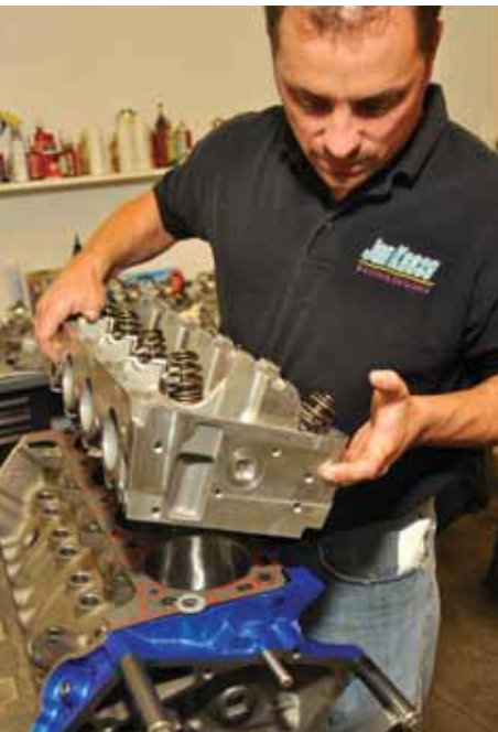
Silicone sealer is applied on both sides and on both ends of the cylinder head gaskets around the oil drain-back holes to ensure a leak-proof seal. Then the cylinder heads are installed
