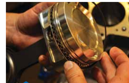
The lower support rail of the oil control ring is installed on the Diamond piston which is followed by the upper support rail, the second ring, and finally the top ring
