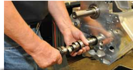
Camshaft specifications vary. Most hot rodders use a hydraulic roller while the racers use a solid roller. For supercharged applications a camshaft is chosen that invariably eliminates jerking and bucking at off-idle and part throttle in the lower gears. For Boss Nine-powered boats a camshaft with wide lobe separation is necessary to ensure a low idle speed. This feature enables easy dock manoeuvring and trailer loading. Note: Aluminium Boss Nine crankcase pictured
