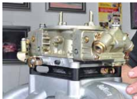
On this Boss Nine a 4150-style four-barrel carburetor sits atop a Wilson Manifolds spacer on a single-plane intake
