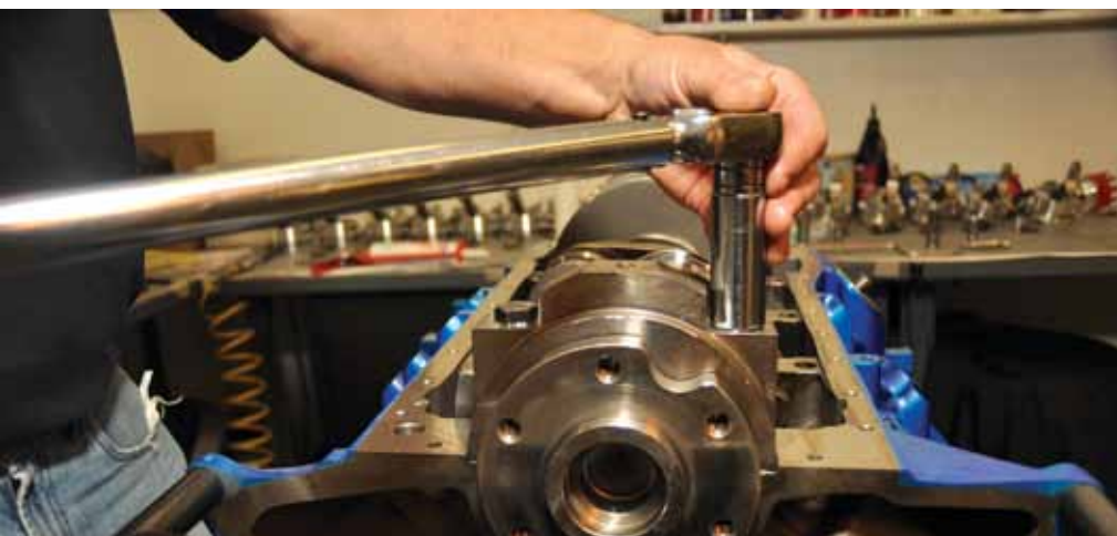
With assembly oil applied to the threads and to under the heads of the 1/2in bolts, the rear main cap is tightened to a torque value of 100lb ft
