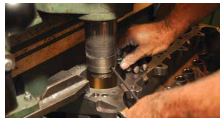
Because cylinder bore dimensions on Boss Nine engines are available from 4.360in and increase to 4.600in, bare block castings arrive with bore sizes usually around 4.340in. Hence the first step in building every Boss Nine engine is boring the engine to almost the designated size. Correct cylinder bore sizes are achieved in the second step, honing
