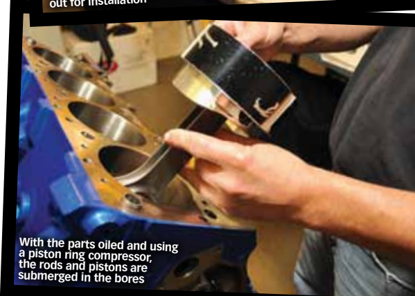
Here the connecting rods have already been assembled in the pistons with Trend H13 tool steel piston pins and set out for installation
