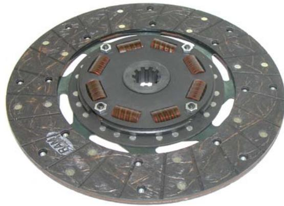
Until the late80s, Pro stock cars used organic friction material similar to that used in today's street cars. For street-strip vehicles, note Ram's urethane encapsulated springs, providing four times increased clutch power.
