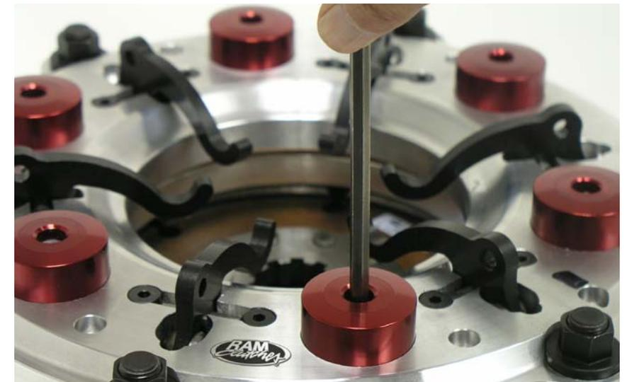
Base pressure is a fixed clamping load that is applied by an Allen key to the top of each clutch spring. Once the gearing is selected, the necessary base pressure and centrifugal weight on the clutch's pressure plate can be determined.
