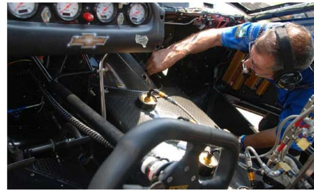
An inspection window at the upper right side of the bellhousing allows crew members access to make final changes to the base pressure and to the centrifugal pressure on the clutch.
