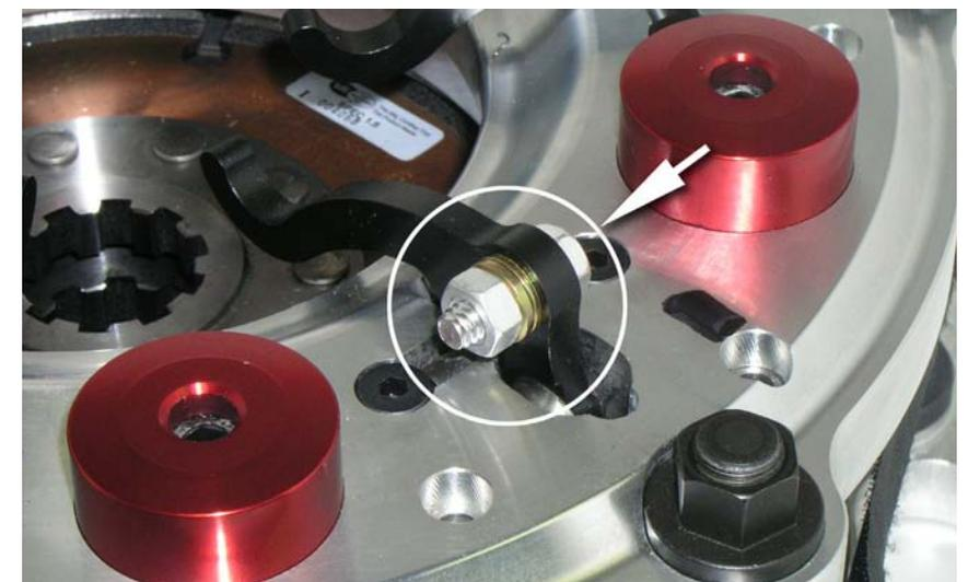
Centrifugal pressure is a variable clamping load applied by engine speed and the weight of a series of small bolts, nuts, and one-gram washers mounted on the clutch fingers.
