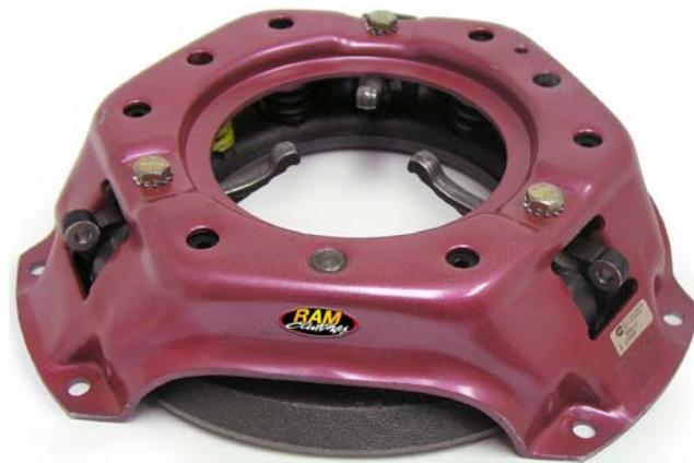
Beefed-up production pressure plates served the Pro Stockers before the universal use of multi-disc racing clutches.
