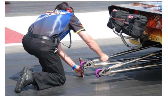
If set correctly, the wheelie bars will break initial traction, helping to promote greater tire speed (wheel spin) at launch. If conditions deteriorate, they may be raised slightly to compensate for reduced traction.
