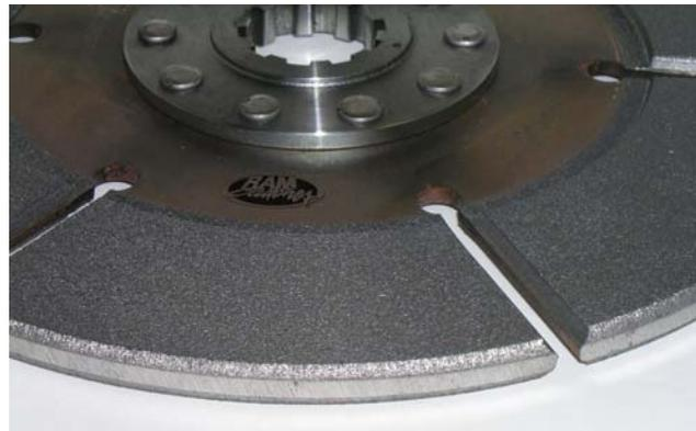
Sintered iron is a powdered mix of different metals bonded to the steel clutch plate and then baked in a furnace.
