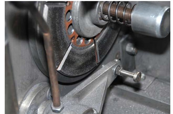
The discs are resurfaced and trued with a diamond-tipped cutter.
