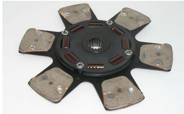
In the early '70s, Ram introduced and patented the paddle disc. It functioned with metallic friction pads, which were later superseded by carbon fiber materials and, finally, by the sintered iron discs of today.
