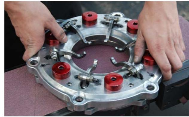
Racing clutch assemblies are serviced after every run. The pressure plate and floater plate(s) are removed and resurfaced, using either a flywheel grinder or belt sander.
