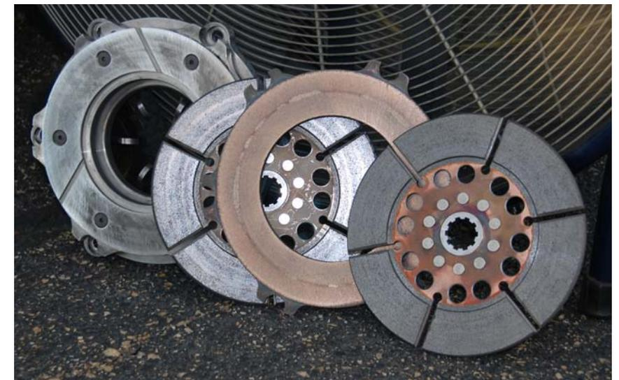
Pro Stock engines transmit their power via a pressure plate (shown on left), two 10-inch clutch plates with sintered linings, and a floater plate that resides between the clutch plates.
